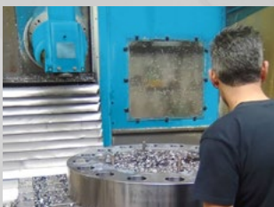
Inhouse machining of CF swivel ring Block 17 Phase 2 Total Angola
