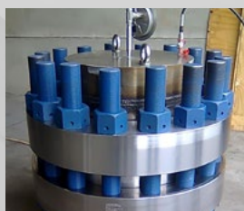
Hydrotest on CF assembly Block 17 phase 2 Total Angola
