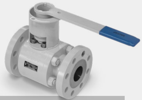
Ball valve with stem extension (for insulation) 2" 300# F321 (-46°C to 160°C)
